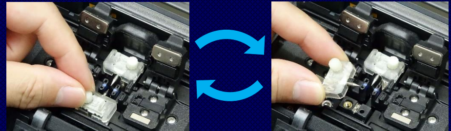
Electrodes replacement without tools
